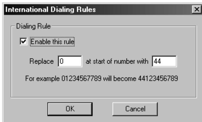
Select 'Enable this rule' to enable dialling rule. Change '44' with the international dialling code for your location. In the example above, the leading '0' will be replaced with '44', e.g. ActiveSMS will convert '07710448818' to '447710123456' before sending a message.
